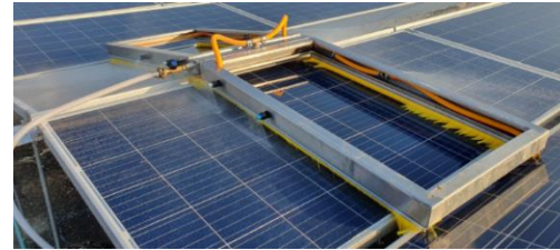
Gal-In manual cleaning system
