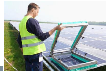
Gal-In manual cleaning system
