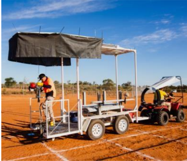
Hammer drill for rod installation
